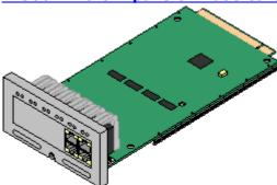
This card adds an additional 4 expansion ports for external expansion modules. The card is supplied with four 2m yellow interconnect cables.
