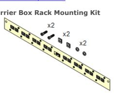
• Barrier Box Rack Mounting Kit (SAP 700293905) Barrier boxes must be used for out-of-building analog phone extensions 36. This bracket allows up to 8 IP Office barrier boxes to be rack mounted and simplifies the number of connections to the protective ground point in the rack. This kit must be used when more than 3 barrier boxes are in use and supports a maximum of 16 barrier boxes for a single external expansion module.
