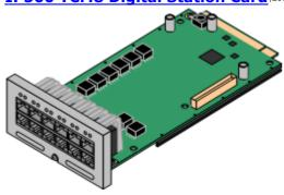
This card provides 8 BST (digital station) ports for the connection of Avaya 4100, 7400, M-Series and T-Series phones.
