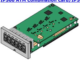
This card provides 6 digital station ports (1-6), 2 analog extension ports (7-8) and 4 analog trunk ports (9-12). The card also includes 10 voice compression channels.
