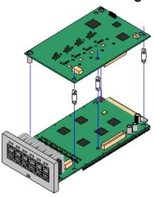
Many IP500 base cards 21h can be fitted with an IP500 trunk daughter cards to support the connection of trunks to the base card.
