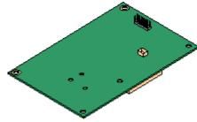
This card allows the base card to support up to 2 PRI trunk connections. The card is available in single and dual port variants. The card can be configured for E1 PRI, T1 robbed bit, T1 PRI or E1R2 PRI trunks. A T1(J) variant for use in Japan is also available.
