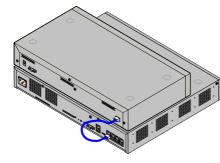
Any external expansion modules should be connected to the control unit before power is applied to the control unit. Ensure that modules are attached in the order that matches the planned or pre-built configuration.
