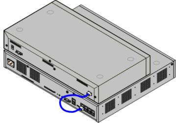
IP500 System with External Expansion Module
