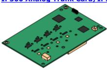
These cards allow the base card to support 4 analog loop-start trunks.
