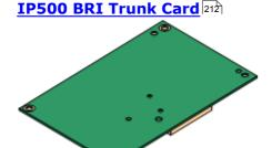
This card allows the base card to support up to 4 BRI trunk connections, each trunk providing 2B+D digital channels. The card is available in 2 port (4 channels) and 4 port (8 channels) variants.
